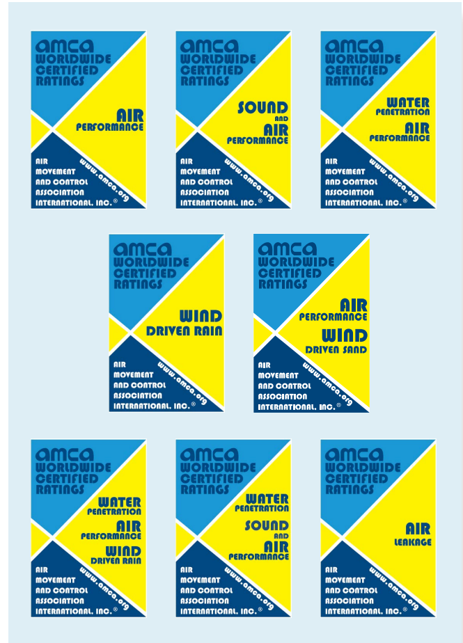
Figure 5. Some of the louver seal types available through the AMCA Certified Ratings Program. Images courtesy of AMCA International.
