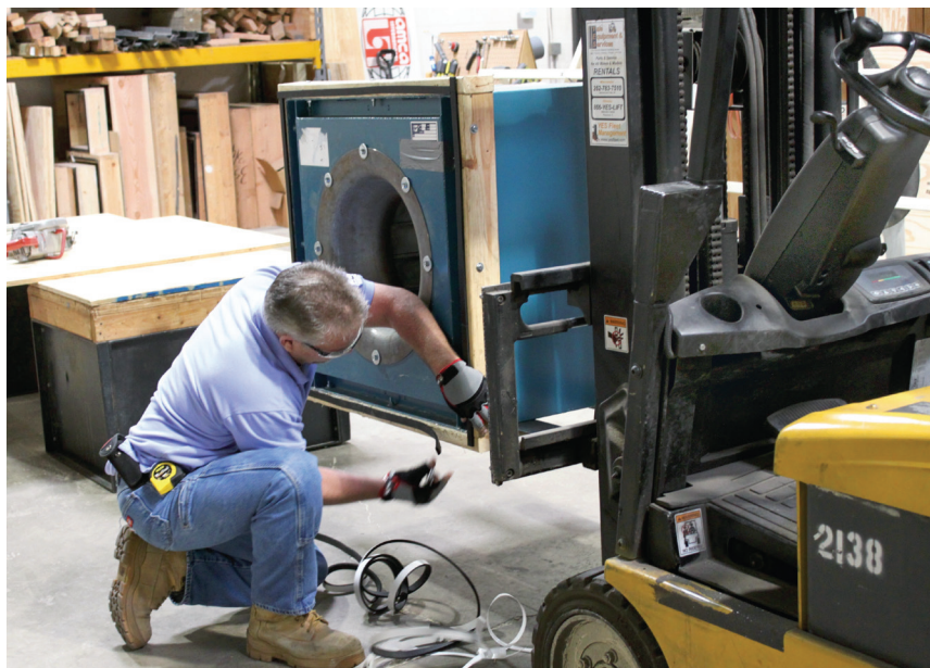
A fan being prepared for testing at the AMCA headquarters laboratory. All photos courtesy of AMCA International.
