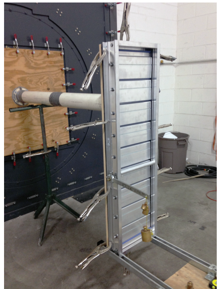
Fan air performance (above) and damper leakage testing (below) at AMCA headquarters laboratory.
